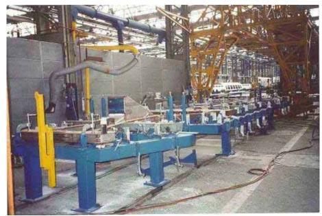
$\begin{tabular}{ll} Figure No. \ 1-SFMTA \ Breda \ Car \ underbody \ structure \ being \ assembled \ using \ the \ assembly \ fixture \end{tabular}$
