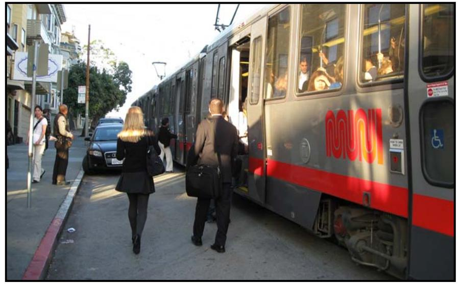
*Carl at Cole Street. Passengers crowd to enter front door or must weave between parked cars to access rear doors of train. Outbound trains have limited visibility due to cars parked on the curve. Illegally parked cars on curve block train or cause side-swipe collisions.*
