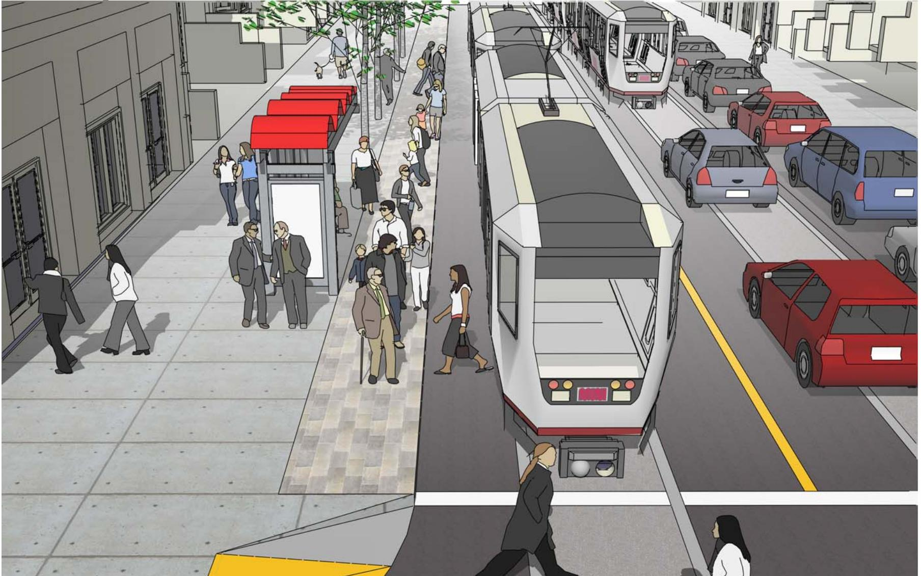
*Sidewalk widened five feet, with a four-foot gap between the train.
