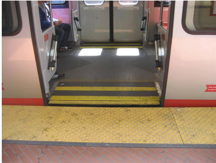
LEVEL-BOARDING PASSENGERS SIMPLY WALK STRAIGHT ABOARD
