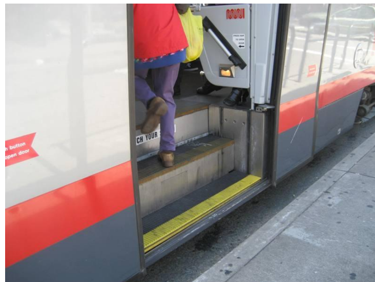
NON-LEVEL-BOARDING PASSENGERS MUST STEP UP TO BOARD
